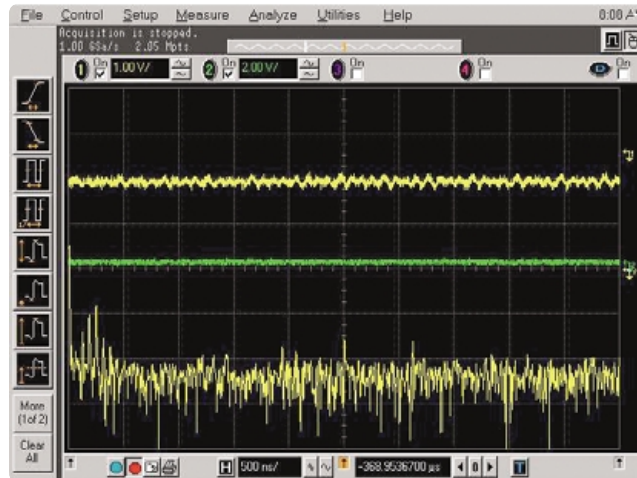
Figure 12. Looking back further in time to the beginning of the baseband transmission, we see noise spikes on the FFT. Some noise spikes are most-likely caused by unintended coupling in the system.
