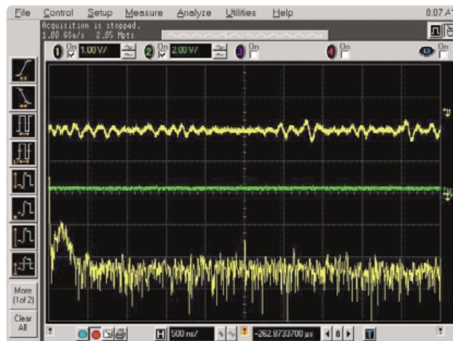
Figure 11. FFT of the Baseband Signal. Most of the energy is located in the leftmost division of the FFT.
